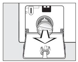
■ Remove the drain filter completely.
